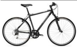
We use Trek 7.3 FX Hybrid 24 speed touring bike with aluminum frame and Shimano gear system.
